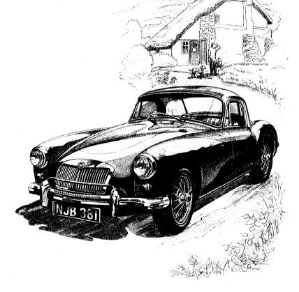
Engine: In-line, 4 cylinder water cooled with a displacement of 1489 cc. Compression ratio: 8.3:1 BHP: 72
