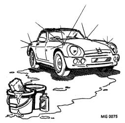
When using a hose, do not direct the jet into the heater air intake ducts, or through the wheels, the brake components, or at the door or window seals, where water pressure could penetrate the seals.
